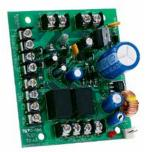
Secured Power Supply Unit – PCB Module
